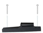
**EACH FOOT**Is mounted to the surface with two screws.
